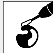
4. Shape the blank with special cutters
