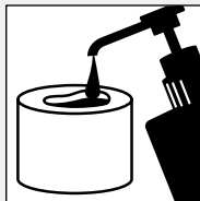
1. Fill the LP material into the transparent negative mold
